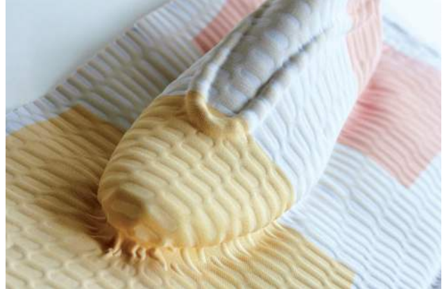
Figure 9: Vacuum forming the uppers of the shoes
